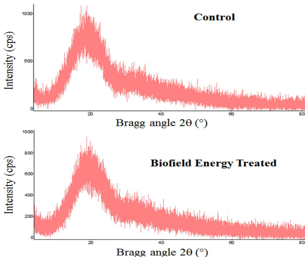
**Figure 1:** PXRD diffractograms of the control and the Biofield Energy Treated PLGA.
