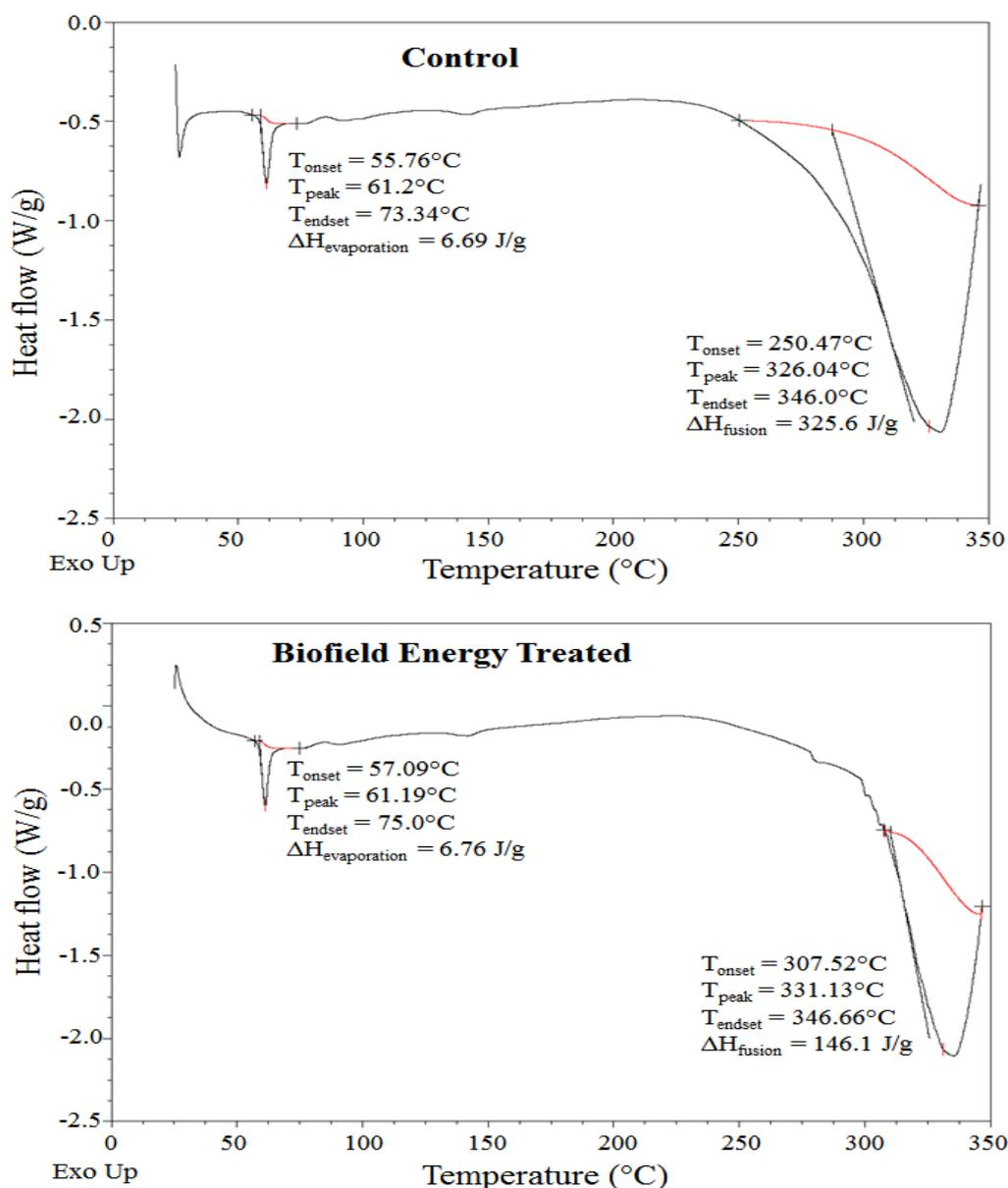
**Figure 2:** DSC thermograms of the control and the Biofield Energy Treated PLGA.
